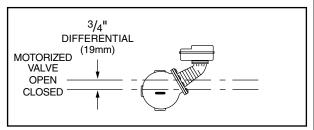
NOTE: Due to the slower operation of some motorized valves, complete valve opening or closing will occur at slightly different levels than indicated above.
