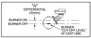
NOTE: Due to the slower operation of some motorized valves, complete valve opening or closing will occur at slightly different levels than indicated above.
