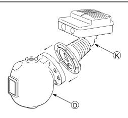
d. Using a wrench, insert the eight (8) bolts and tighten them to approximately 14-20 ft•lb (19-27 N•m) in an alternating star pattern.
