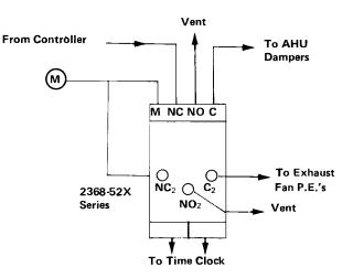
In the application shown, if the fan starts when the time clock contact is closed (day), the controller modulates the air handling unit dampers and the building exhaust fans are started. When the fan is stopped and/or the time clock contact is open (night), the air line to the unit dampers is vented along with the air line to the exhaust fan PE, allowing the unit dampers to close and stopping the exhaust fans.
