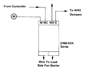
In the application shown, when the fan is started, the relay switches "C" to "NC" and the controller modulates the air handling unit dampers. When the fan is stopped, the relay switches "C" to "NO" and the air line to the dampers is vented.
