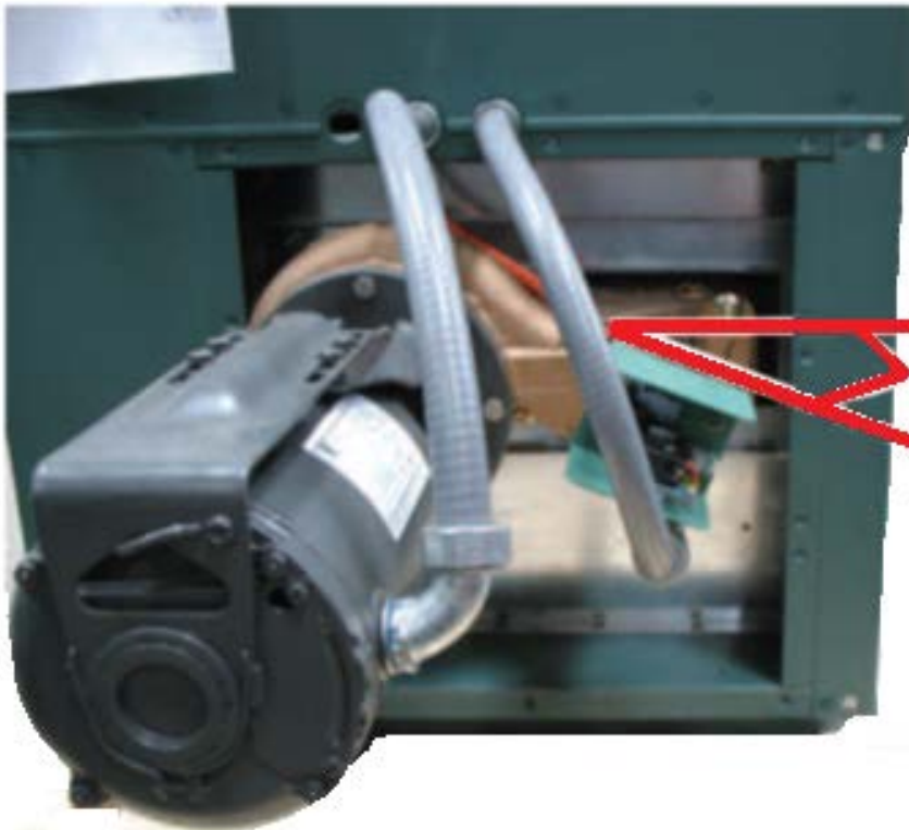
HI-DELTA Models 992A,B & C – 2342A,B & C with Integral Pump Flow switch must be tilted 25^{\circ} \pm 5^{\circ} From Horizontal
