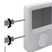
Step 6. Snap into place and tighten mounting screws.
