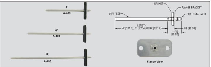
The Stainless Steel Static Pressure Tips are used to measure static pressures in ducts or rooms. They are to be connected to differential pressure switches and transmitters. Two static sensors are used in applications where differential pressure is required across a filter or coil. These sensors include a mounting flange with integral rubber gasket and two screws for simplifying mounting on a duct.
