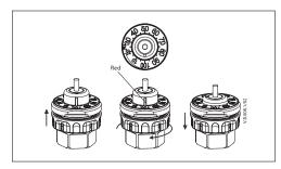
Required flow from  $\frac{1}{2}$ " to  $\frac{1}{4}$ " is easily adjusted without special tools:
