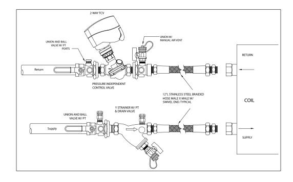
The AB-QM is a versatile device that can be used as an actuated or non-actuated balance valve / flow limiter. With an actuator mounted to the AB-QM valve, the assembly is a pressure independent control valve. Utilizing a proportioning controller, the AB-QM creates a robust and stable energy management sub system using only the required flow and energy to offset facility heat transfer gains and losses.
