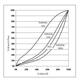
The interaction of  $\Delta P_{SYSTEM}$  on the control valve can significantly hinder the control valve's effectiveness. The design of the AB-QM's internal differential pressure regulator address this by counteracting the inlet  $\Delta P_{SYSTEM}$  fluctuations, and as a result a constant differential pressure across the control valve is achieved.
