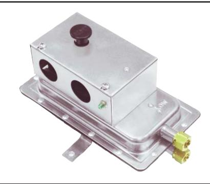
mounting with the sample line connections in the "up" position. Surface mount via the two 3/16" (4.75 mm) diameter holes in the integral mounting bracket. The mounting holes are 3-7/8" (98.4 mm) apart.
