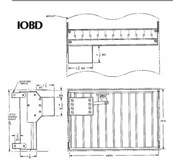
Wire damper motor first snaking wire thru duct and then insert damper into duct opening and secure with self-tapping screws (provided) thru mounting tabs.
