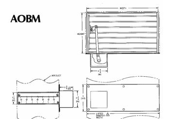
Cut a 3" slot in the bottom of the duct, slide the damper in and secure with self-tapping screws provided.
