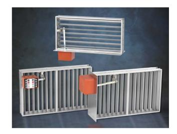
The MST motor powers the damper open and closed and is designed to operate in all weather conditions. The AOBD is recommended for low pressure duct systems, less than 0.75" S.P. For higher pressure systems use the Comfortron series of dampers.
