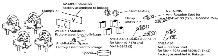
\* Clamp blocks are only required for the MX41-634x and Mx40-717x actuators.
