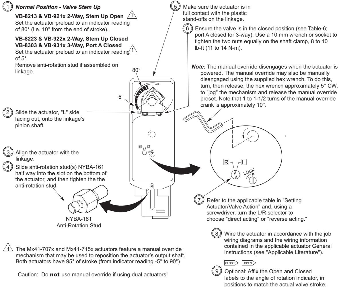
**Figure-4 Mounting Mx41-707x or M41-715x and Setting Up Actuator/Linkage/Valve**
