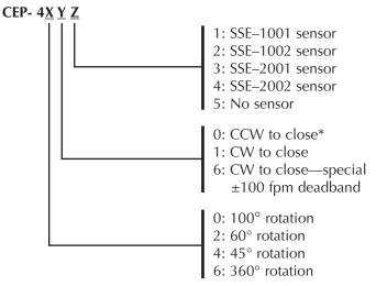
**\*NOTE:** The default rotation direction can easily be reversed by swapping the red and blue motor wires.
