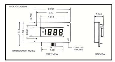
The remote mounting from the PC board allows you to provide a custom look to your control panel, while still using a standard product. The mounting is a simple bezel arrangement.
