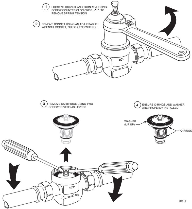
Fig. 2. Replacing D05T cartridge.
