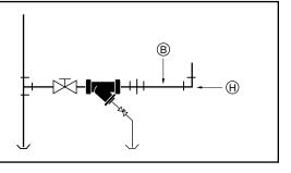
**3.** Position the bucket trap so that the cover (J) is on top and the inlet pipe (B) will connect with the bottom inlet tapping (K).
