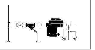
If the gate valve (M) is not connected to a drain, install a cap (P) on the outlet pipe (N).
