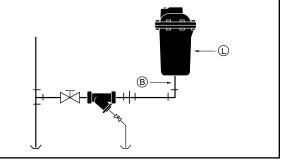
Remove the 1/2" (15mm) pipe lug (L) on the trap cover (J).
