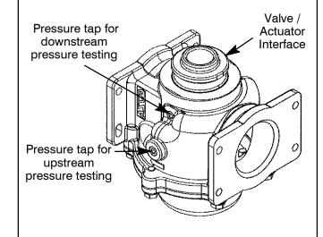
Note: Upstream and downstream pressure taps are on either side of valve body.
