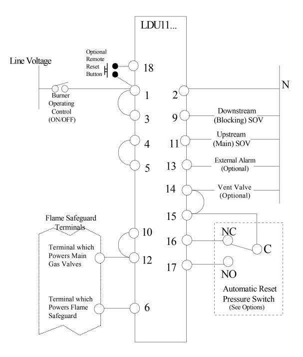
Below is the wiring diagram using a LFL flame safeguard performing the leak test before burner start-up and after a controlled shut-down. This diagram only depicts the wires that are connected to the LDU control. Please consult Siemens manual 7451 for further wiring instructions for the LFL burner control.
