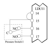
During Test 1, power is on Terminal 15. After the area between the gas valves has been evacuated of pressure, the switch should have power through terminal 15 to terminal 16. If the main gas valve is leaking, the area between the gas valves fills with gas, leak detection pressure switch I trips, sending power to terminal 17, causing a lockout.
