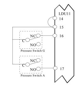
During Test 1, Terminal 15 is powered. After the area between the gas valves has been evaluated of pressure, pressure G switch should have power through terminal 15 to terminal 16. If the main gas valve is leaking, the area between the gas valves fills with gas, pressure switch A trips, sending power to terminal 17, causing a lockout.
