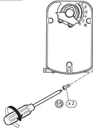
15. Tighten bracket screws.
