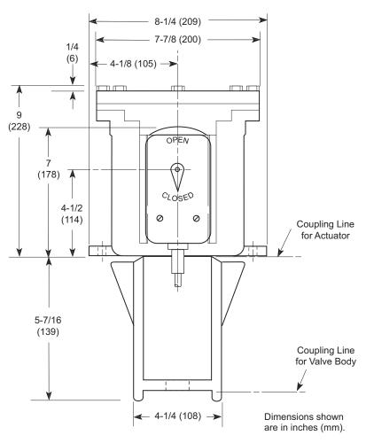
Allow 12" (300 mm) minimum service clearance above the housing top.
