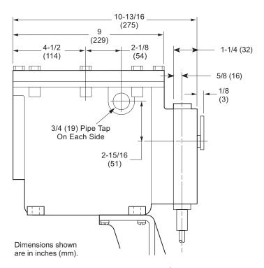
Figure-10 Hazardous Location Actuator Side Dimensions.
