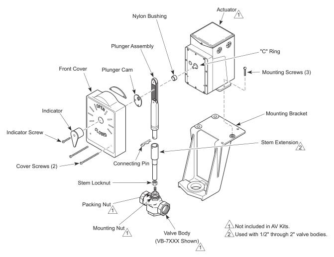
Figure-4 Components for Valve Installation of Standard Actuator.
