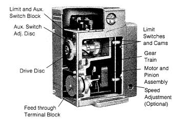
Figure-7 Cut-a-way of Actuator.
