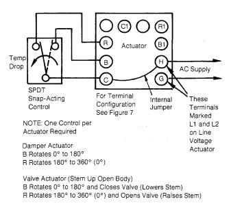
Figure-2 External Wiring for Heating Application.
