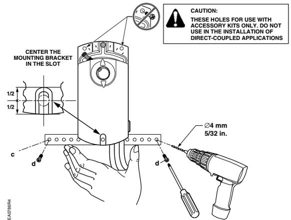
Figure 9. Attaching the Anti-rotation Bracket.
