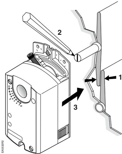
Figure 7. Mounting the Actuator to the Damper Shaft.
