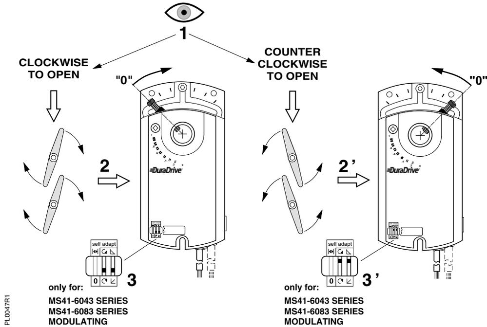
Figure 3. Setting the Direction of Rotation.
