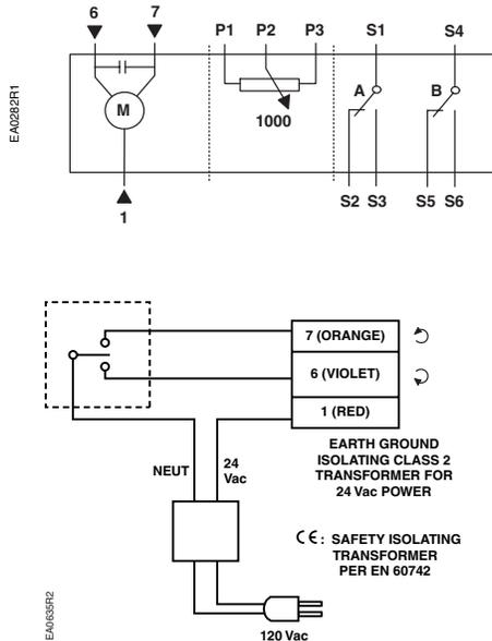
Figure 15. Three-position Control.
