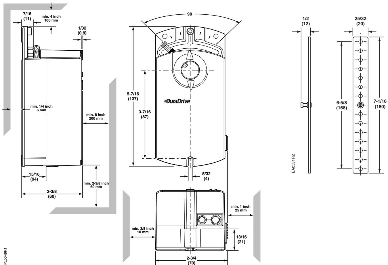
Figure 17. Dimensions of TAC DuraDrive Actuator and Anti-rotation Bracket.
