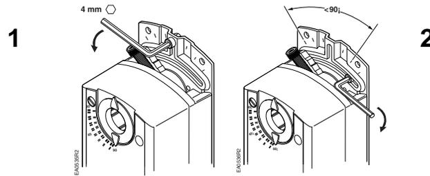
Figure 12. Moving the Mechanical Range Stop.
