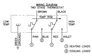
THERMOSTAT OPERATION: DOUBLE POLE, DOUBLE THROW CONTACTS OPERATE SEQUENTIALLY WITH 3'F (1.7'C) NOMINAL SEPARATION ON TEMPERATURE RISE OR FALL. AT TEMPERATURE ABOVE THE SET POINT, LEADS BLACK/VIOLET AND BROWN/BLUE ARE CLOSED. ON TEMPERATURE FALL TO 3'F (1.7'C) (NOMINAL) ABOVE THE SET POINT, LEADS BLACK/RED CLOSE AND BLACK/VIOLET OPEN. ON FURTHER TEMPERATURE FALL TO THE SET POINT, LEADS BROWN/PINK CLOSE AND BROWN/BLUE OPEN.
