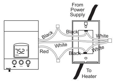
Attach wires per diagram above. Note:
