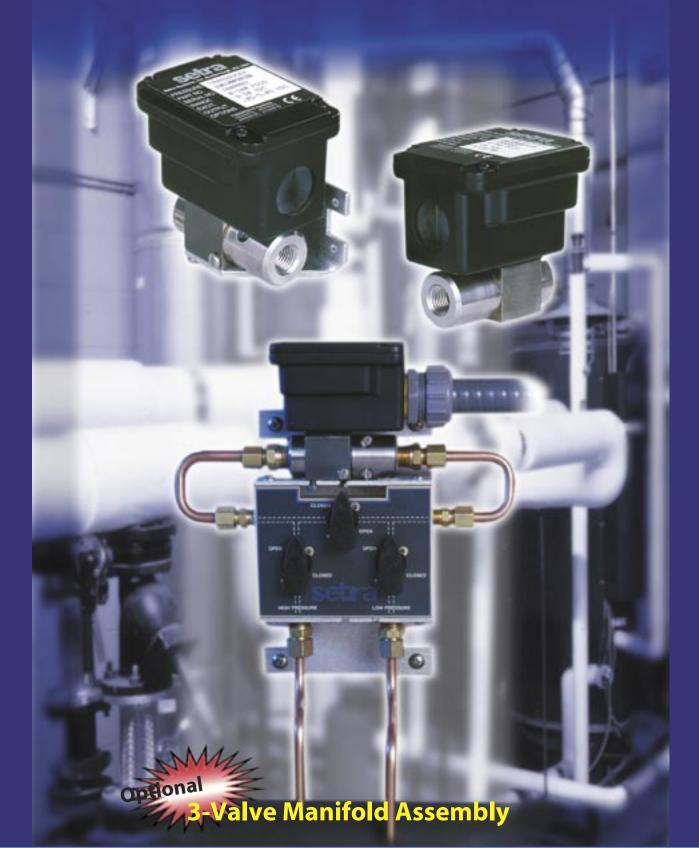
Setra Systems Model 230 is a high output, low differential pressure transducer designed for wet to wet differential pressure measurements of liquids or gases. A fast-response capacitance sensor and signal conditioned electronic circuitry provide a highly accurate, linear analog output proportional to pressure. Both unidirectional and bidirectional pressure ranges are available for applications with line pressure up to 250 psig.
