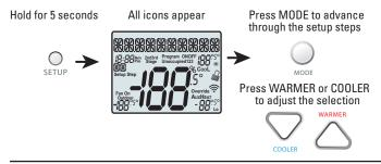
Technician Setup is for diagnostic and testing purposes and is intended for use by a qualified technician. See page 14 for more detailed instructions.
