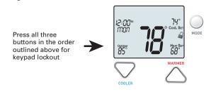
To *unlock* the keypad, press and hold the MODE button. While holding the MODE button, press the WARMER and COOLER buttons together. The icon will disappear from the display, then release the buttons.
