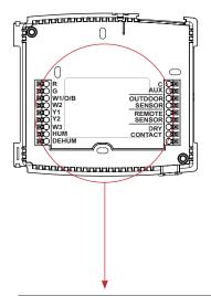
To remove the thermostat backplate: Gently separate the display from the base by pulling first from one side, then the other until the two pieces unsnap. A small screwdriver may be used, very carefully, to start seperating the two pieces.
