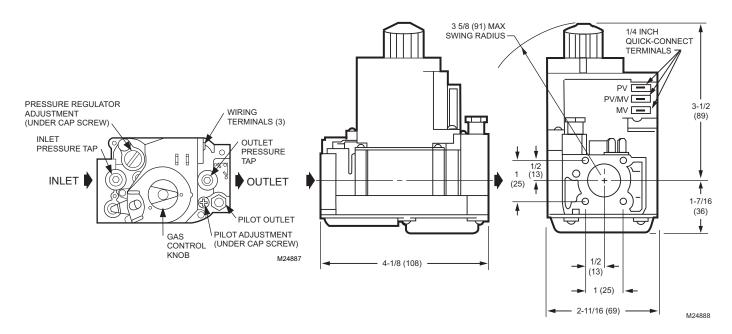
Fig. 4. VR8204A mounting dimensions in inches (mm).
