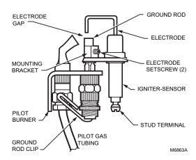
Fig. 9. Fasten igniter-sensor to ground rod.
