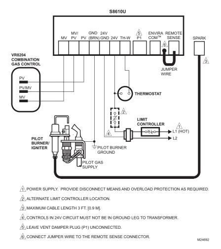
Fig. 16. Y8610U connections in a heating system with an atmospheric burner and no vent damper.
