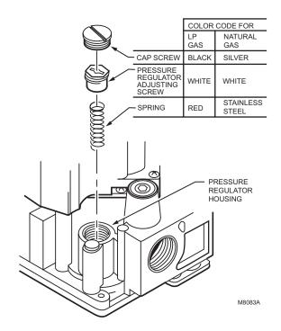
Fig. 10. Installation of conversion kit in regulated gas control.
