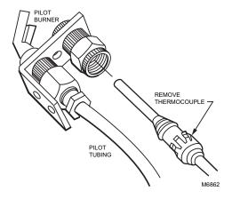
Fig. 7. Remove thermocouple from pilot burner.
