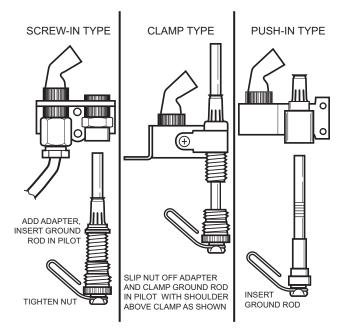
Fig. 8. Mount ground rod on pilot burner.
