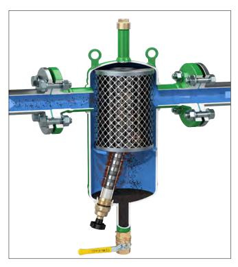
To purge the debris, the flexible magnetic stack is removed from the brass dry-well and, even while the system is still running, the drain valve is opened. Aided by the system pressure, the dirt and magnetite flushes out quickly and effectively. DIRTMAG® magnetic dirt separators accomplish  $2\frac{1}{2}$  times the ferrous impurities removal performance of standard dirt separators, delivering up to 100% elimination efficiency.
