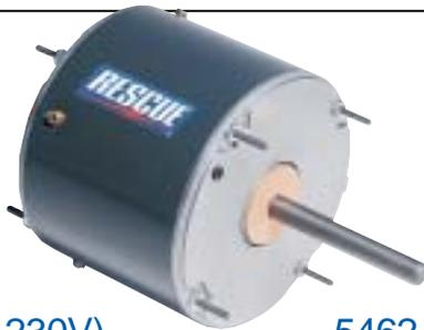
Features: 48 Frame, 5.6" Diameter, 60°C Ambient Rated, All Position Mounting, Ball Bearings, Totally Enclosed (air over), Reversible, Rheem Mounting Holes
