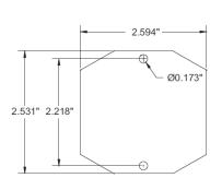
Mount the octal socket (base) on rigid vertical or horizontal surface using #6 or #8 screws. The control should be mounted within an enclosure of proper NEMA integrity.
