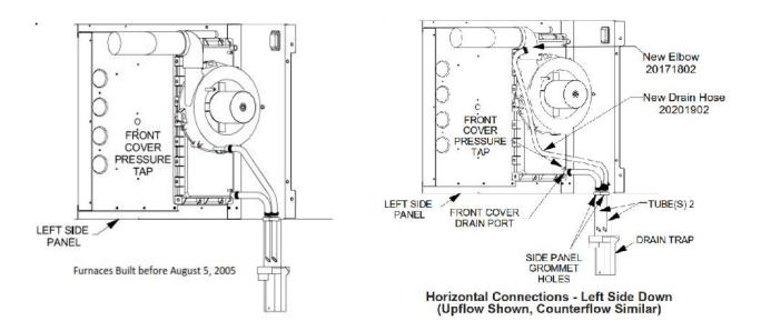
For furnaces using the alternate flue connection in the horizontal left position, you can use the RF000142 kit and follow the instruction provided in the kit.
