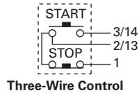
When more than one pushbutton station is used, omit Connector "A" and connect per sketch at right.
